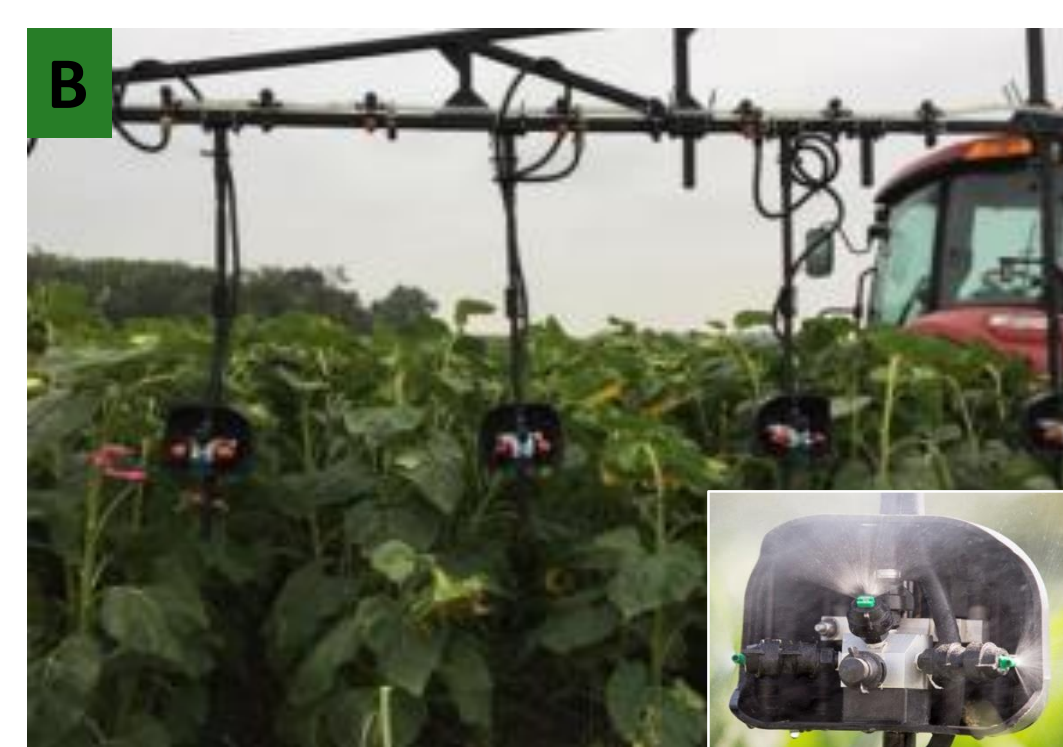
Figure 2b. Ground rig equipped with 360° Undercover™ drop nozzle for beneath canopy application to sunflower face. Photo credit: USDA-APHIS-WS NWRC
