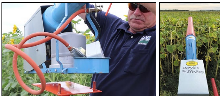
Figure 125. A gas exploder, when properly located and moved within the field every two to three days, can reduce bird damage.
